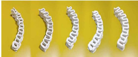
Fig. 6 Different nozzle sizes
