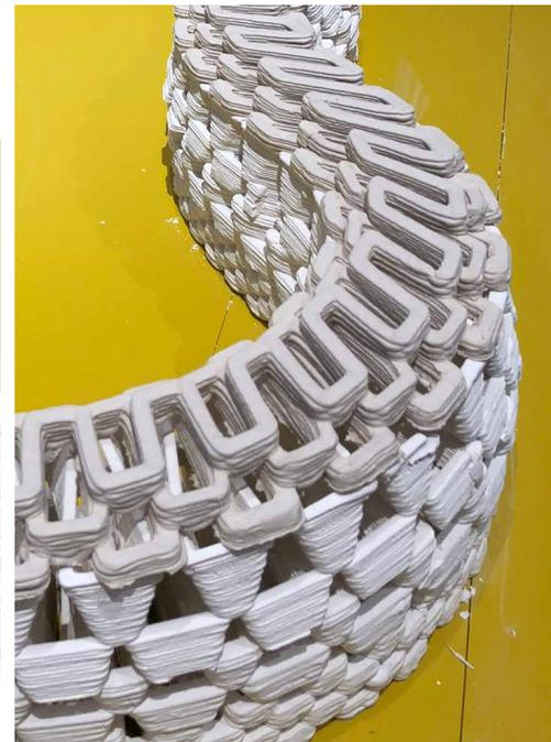
Fig. 10. Shifted layer setup with varying thicknesses
