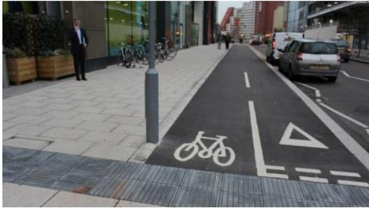
**Fig. 4:** The tactile pavement system to highlight the border with the cycle lane.
