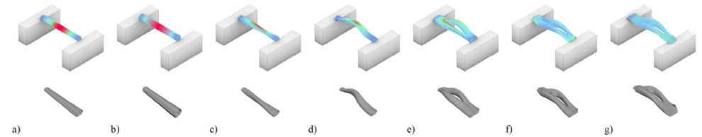
**Figure 1.** (a-g) Design sequence and structural evaluation of a series of options for a 3d printed pedestrian bridge. Bottom row shows the designed geometry; top row shows structural evaluation diagram of each of the options. Red colors signify larger deflections in geometry while green and blue identify a more stable shape.
